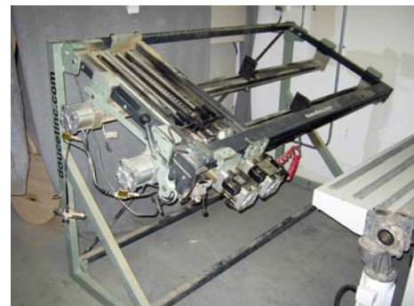
2008 Doucet Door Clamp (MSU142) for mitre and stile & rail cabinet doors.
