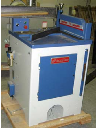
AccuTek 18" pneu. chop saw (MSL518) 10 hp main motor, 2" x 12" capacity.
