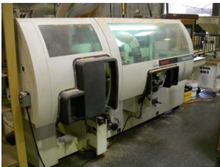
2000 SCM Superset Moulder (MSU136) 5 spindle, plus universal.
