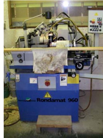
2006 Weinig R960 Grinder (MSU135) For HSK & conventional heads.
